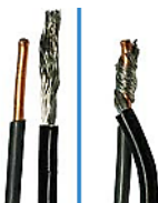
Figure 3-26 Strip Ends and twist
